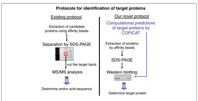
Figure 1 Schematic illustration of our protocol combining in silico screening and experimental verification for identification of target protein.
